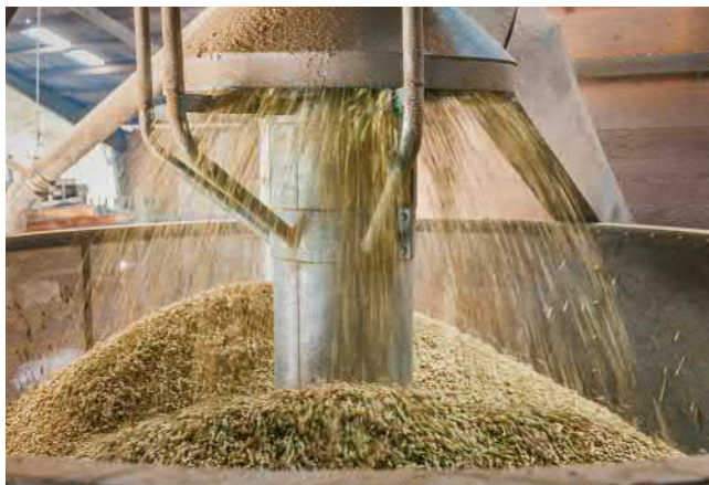
Modern kiln for unripe spelt with drying tower
